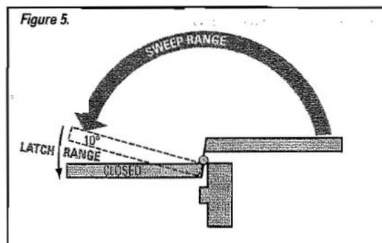
**Backcheck** controls the Opening of the door by slowing it down as it approaches fully opened position—it keeps the door from slamming open. It's desirable for three reasons: it reduces the hazard to people who may be struck by the swinging door, it reduces the possibility of damage to the door or adjacent wall, and it reduces the stress on door hardware.
