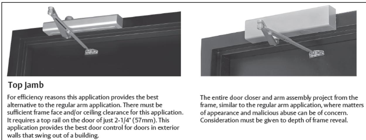
In a Top jamb installation the length of the arm is determined by the distance from the face of the closed door to the face of the frame (the reveal). A deep reveal will need a long arm.
