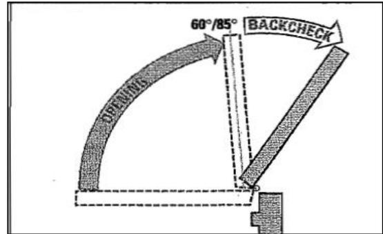
A **Delay Range** is an optional control that holds the door open for a short period of time before beginning the closing cycle. Delayed Action provides more time to move through the opening before the door begins to close, and is useful when there is frequent traffic from carts, dollies, wheelchairs, or slow-moving people such as the elderly or children. Typically the Delay period is adjustable to suit the needs of the occupants.
