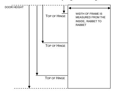
Since hinges vary in size, the dimension from the edge of the hinge to the centerline of the hinge is determined and added to the top-of-hinge dimension to get the placement for the template.
