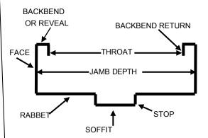
**backbend:** the edge of the frame bent 90° from the face toward the wall material, provides rigidity
