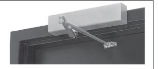
The entire door closer and arm assembly project from the frame, similar to the regular arm application, where matters of appearance and malicious abuse can be of concern. Consideration must be given to depth of frame reveal.
